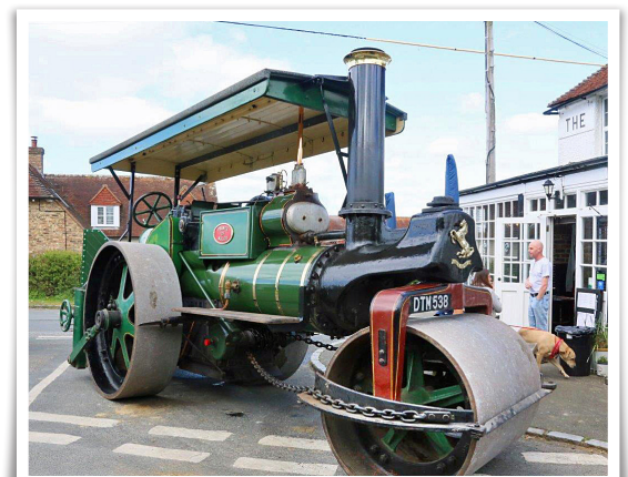
Aveling Barford W class roller 10 tons. Single cylinder with piston valve gear. 1937, 'Prince of Wales'. Peter Love
